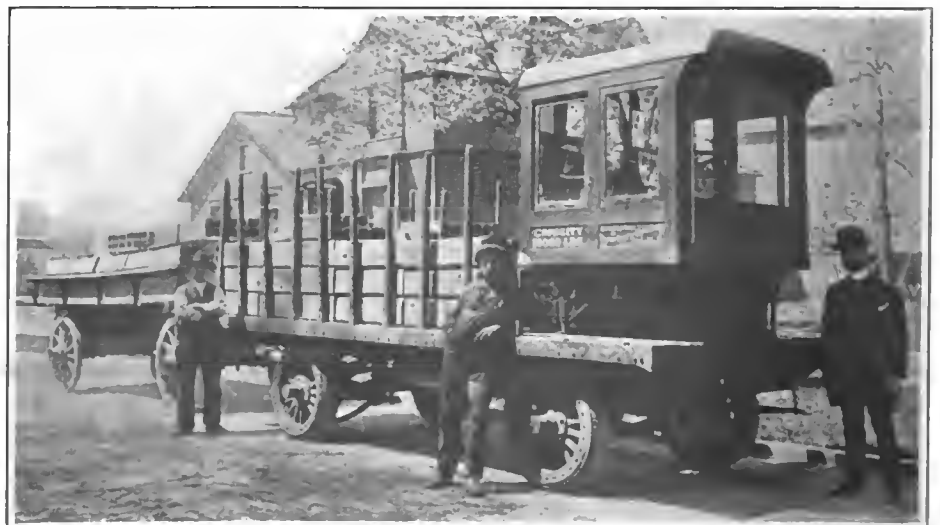
WHITING CONVERTIBLE GASOLINE TRUCK, WITH LOADED TRAILER BEHIND.
